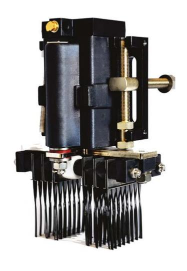
Operated by a signal from the driver's cab, the Rail Brush works by compressed air entering the cylinder to extend the brush down on to the rail. The force and scraping action of the tines cleans the rail and, when required, the Rail Brush retracts and springs fully clear of the rail in response to the signal from the cab being removed. The brush head is designed for quick trackside replacement with minimum downtime.
